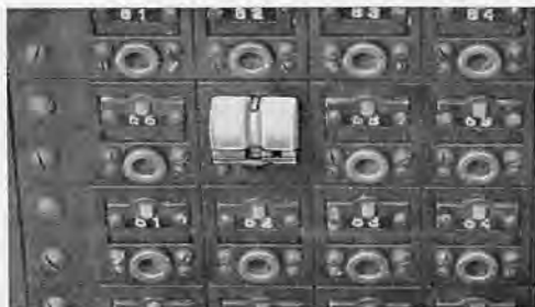
Fig. 10—Appearance of No. 11 Type Drop shutter when viewed from above.
