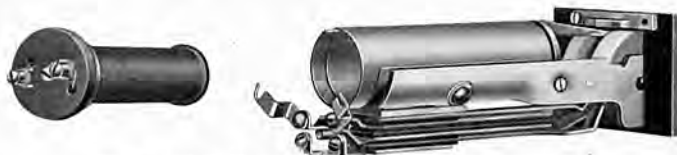
Fig. 5—Coil Removed and Leads Disconnected
