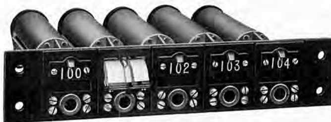
Fig. 3—Front View, Bank of No. 11 Drops
