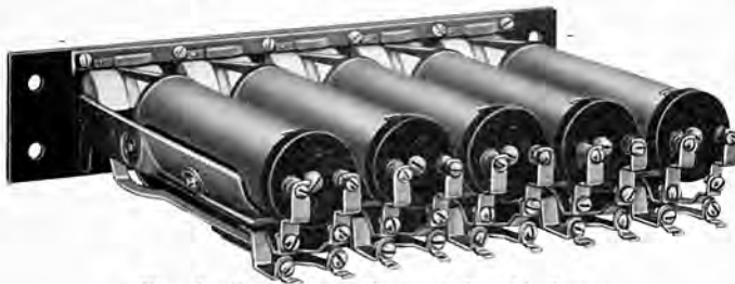
Fig. 4—Rear View, Bank of No. 11 Drops
