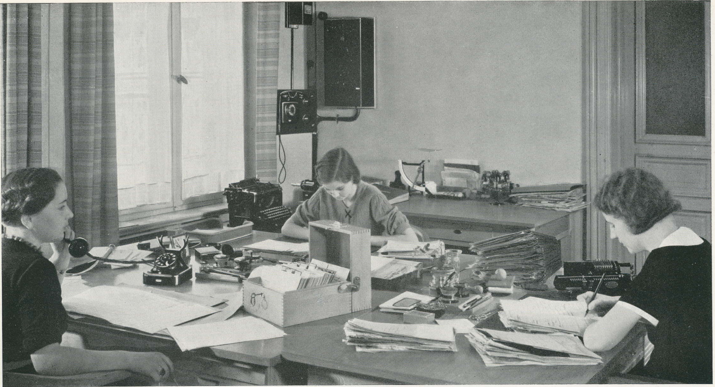
NEHA exchange for 1 exchange line and 10 extensions with central station
