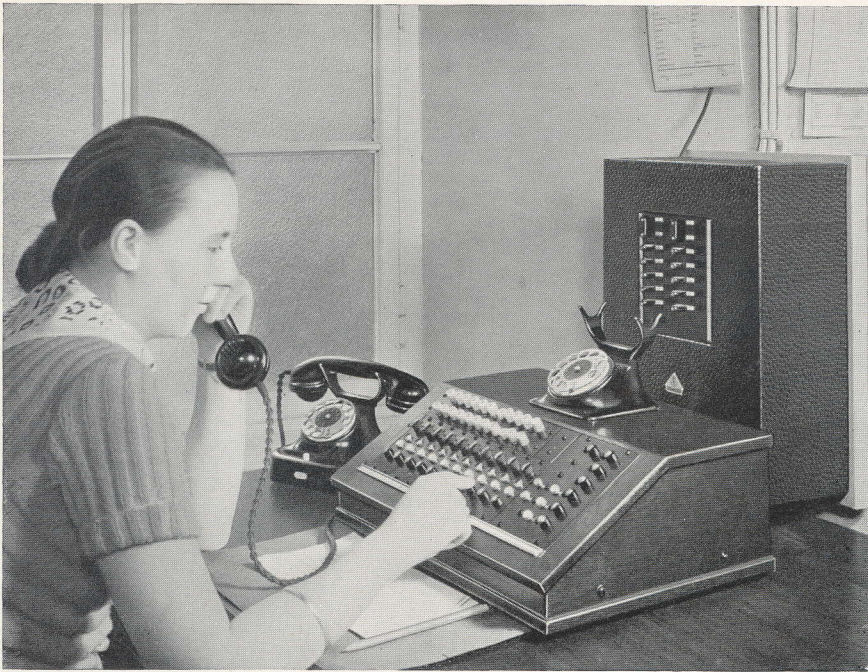
NEHA Private Exchange for 10 exchange lines and 90 extensions
